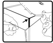
Remove top cover and perspex sides. (Note: perspex corner to be aligned with black corner of unit when re-fitting.)
