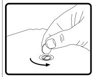
Undo top cover screw using a 5¢ piece, key head or screw driver. Only 1/4 turn is needed.
